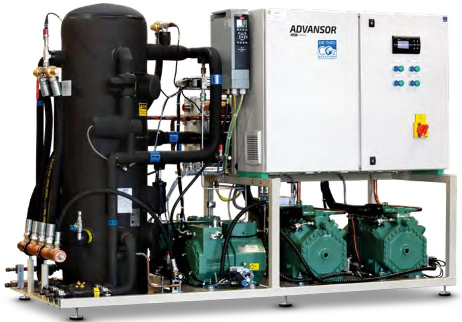
Simple and compact designed, yet very easy to service. Suits every medium size supermarket or industrial applications with a wide range of options. The design is optimized with compressors in only one layer, the electrical panel above and the receiver left to the compressors. Combined with the use of K65 piping, this leads to a very simple and compact design.
