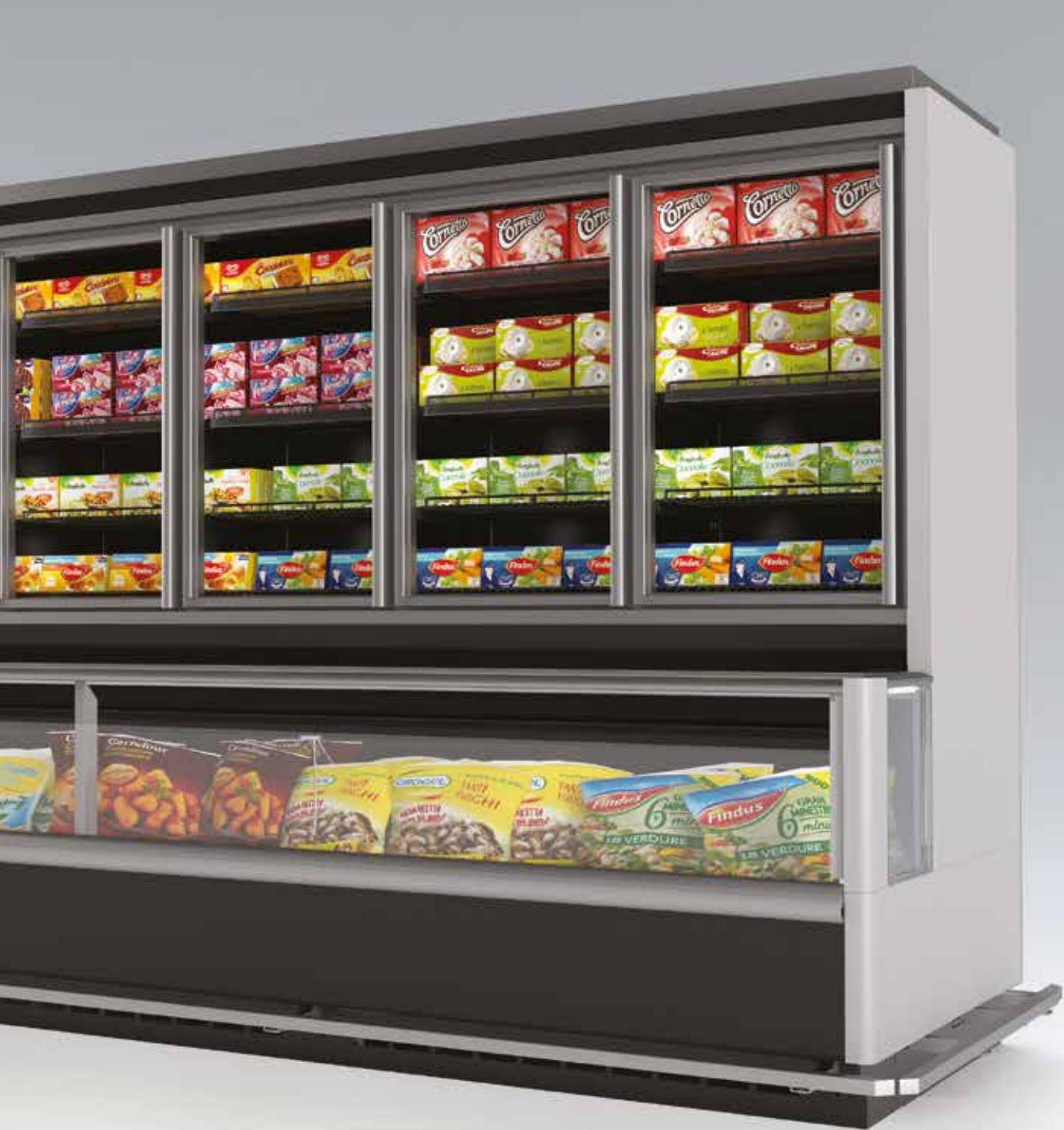
**TASMANIA 2.0** is a combined vertical unit with a deck and an upper section with doors, designed for two display needs: packaged meat (class M1) and/or frozen items and ice-cream (class L1) in the lower part, while the upper section is dedicated to frozen products and ice-cream (class L1) only. It comes in 2 heights: 2060 and 2180mm.
